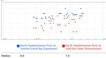
River pH is measured using Hach kits that compare a change in water color.
