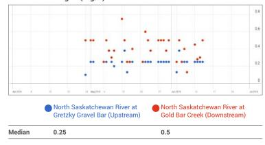
Ammonia nitrogen concentrations are measured by dipping Hach test strips into water and noting the color change
