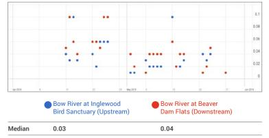
$Ammonia\ nitrogen\ concentrations\ are\ measured\ by\ dipping\ Hach\ test\ strips\ into\ water\ and\ noting\ the\ color\ change.$
