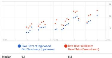
Dissolved oxygen concentrations are measured using Hach kits with a drop-by-drop titration to show a change in water color until totally clear. Dissolved oxygen is tested during daylight while macrophyte and algae photosynthesis is underway and generating oxygen. The first upstream test site is sampled in the morning; the second downstream test site is sampled in the early afternoon.
